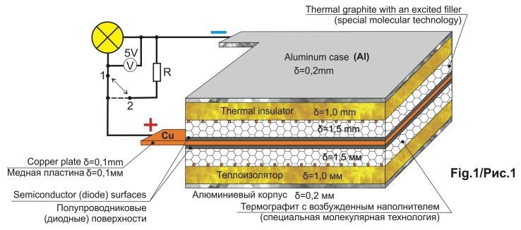
The thickness of the "sandwich» S=2(0.2mm+1.0mm+1.5mm)+0.1mm=5.5mm
